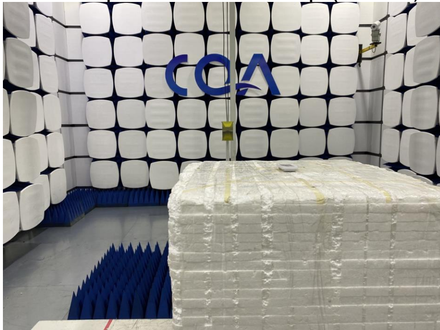
Radiated spurious emission Test Setup-2(Above 1GHz)
